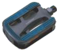
PDL-002 Material: Two-Pieces PP with Inlaid TPR Tread Non-Slip Size: 97*73mm
