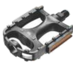
PDL-003 Material: Two-Pieces PP with Inlaid TPR Tread Non-Slip Size: 97*85mm
