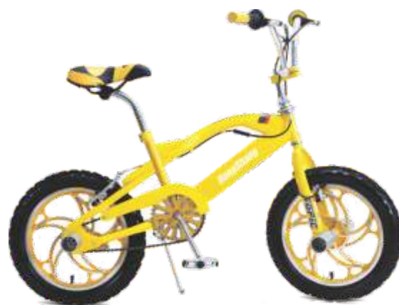
FSB-201 Frame: Steel Mig Welded Fork : Steel 16" without Pivot Tyre : 16" x 2.125 Brake : Caliper Brake
